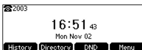
The idle screen displays the label of the current account, time and date, and four soft keys.
