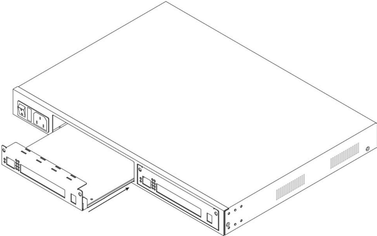
**Figure 5-4 Installing a Network Module into the IES-1000 Chassis**
