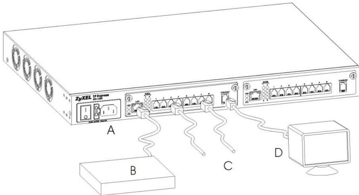
**Figure 6-1 SAM1008 Front Panel Connections Overview**
