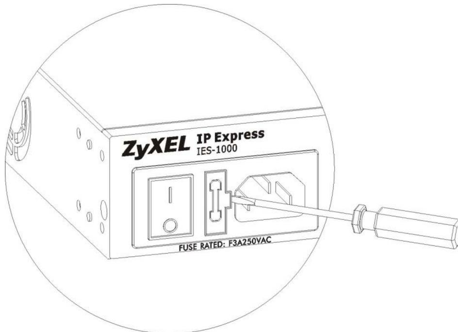
**Diagram 1 Opening the Fuse Housing**
