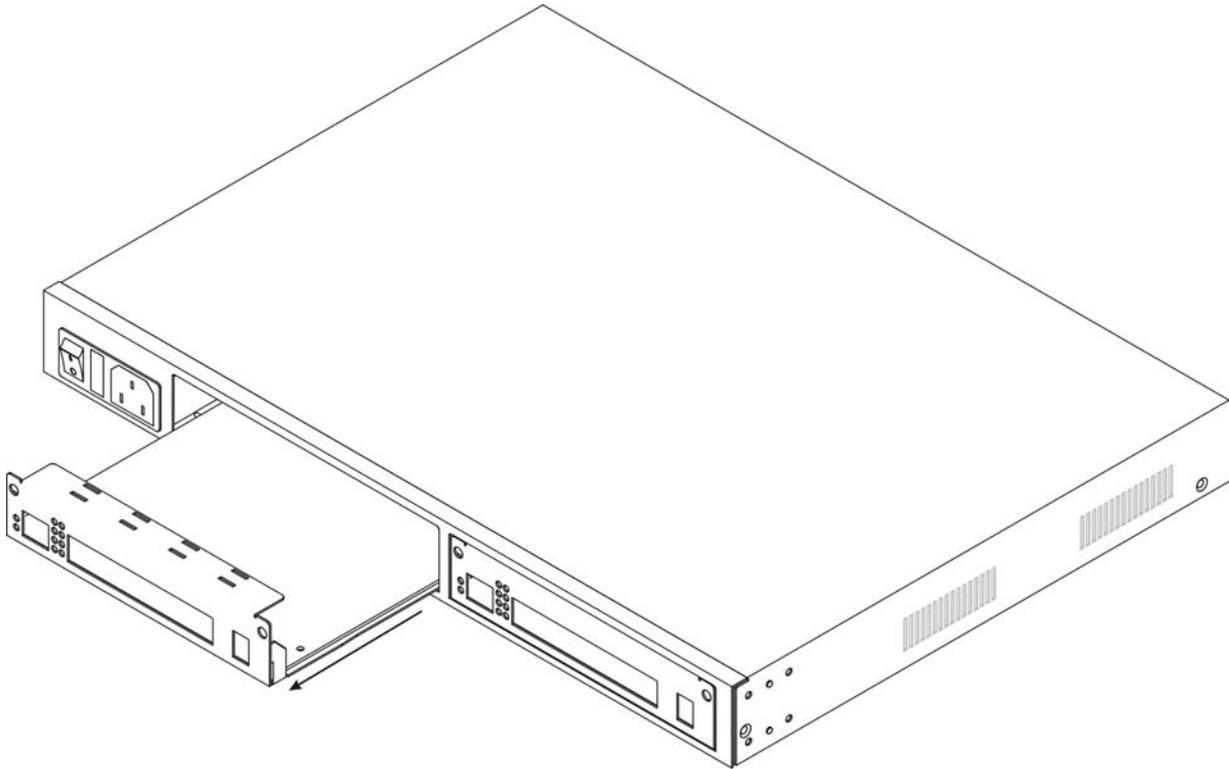
**Figure 5-3 Removing a Network Module from the IES-1000 Chassis**
