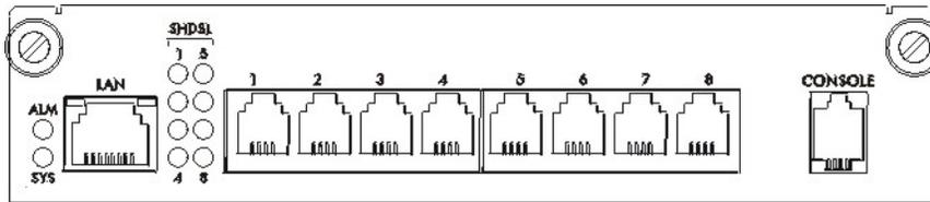
Figure 7-2 SAM1008 Front Panel LEDs
