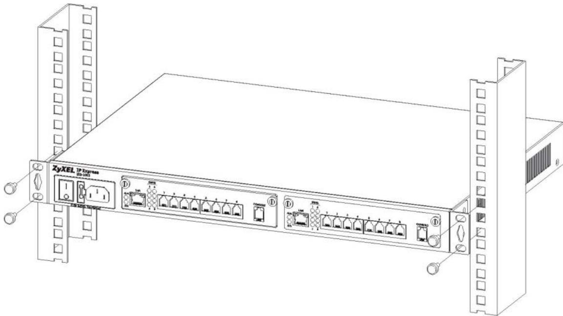
**Figure 4-2 Mounting the IES-1000 on a Rack**
