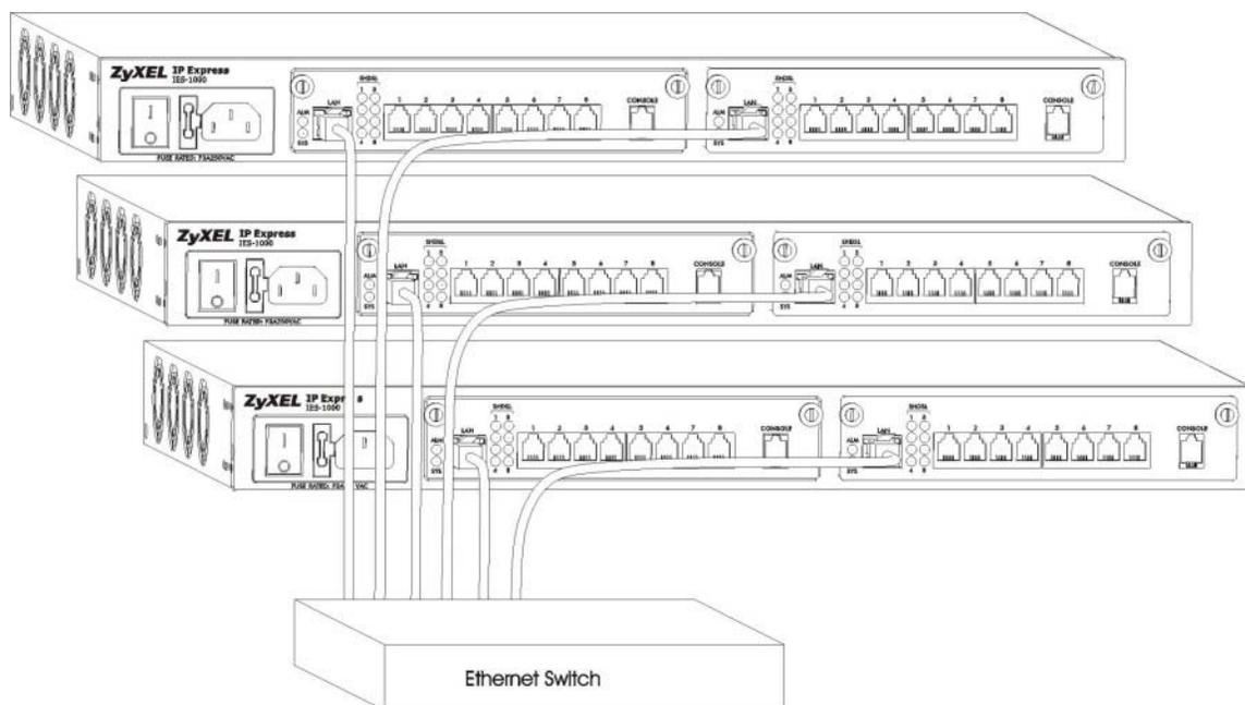
Figure 6-12 Stacking Multiple IES-1000 Units
