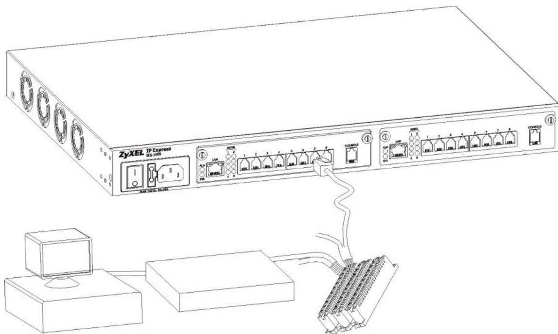
**Figure 6-4 SHDSL Port, MDF and User Equipment Connections**
