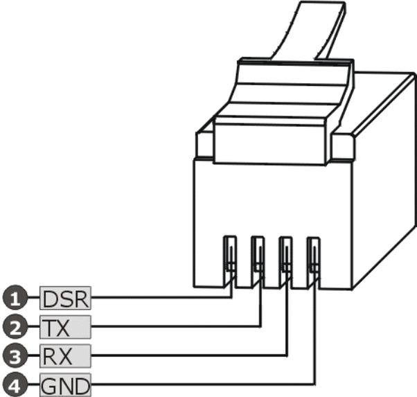
Diagram 3 RJ-11 4P4C (Console Port) Pin Assignments
