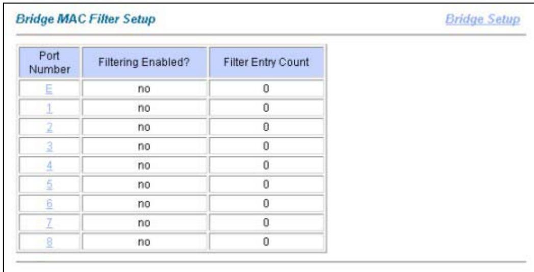
**Figure 10-7 Bridge MAC Filter Setup**
