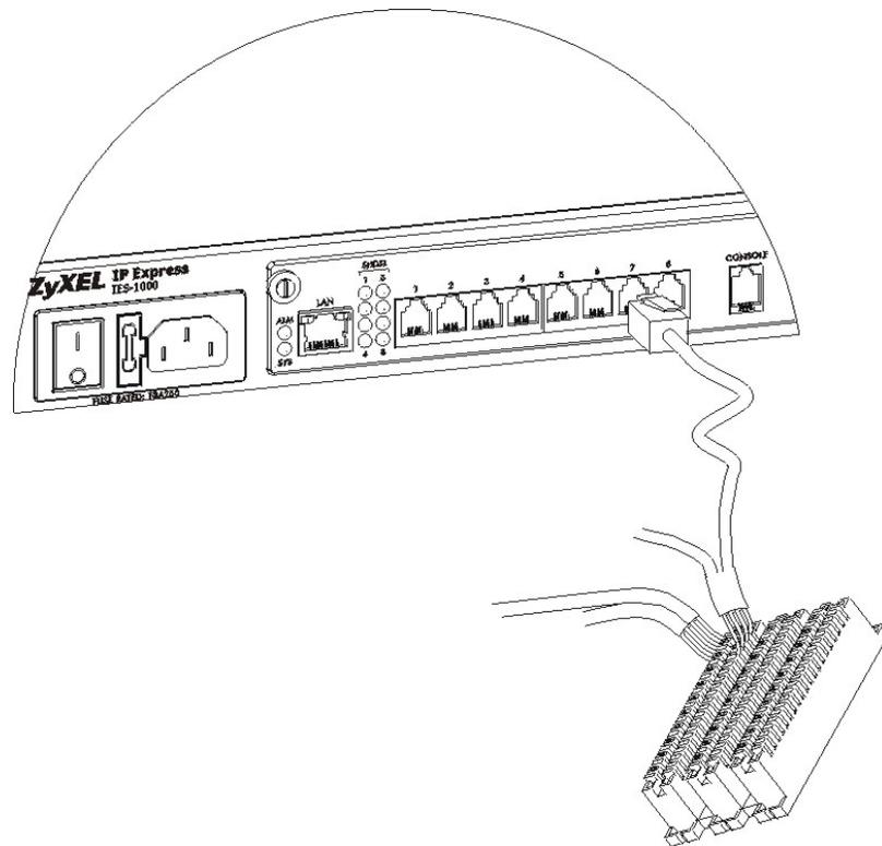
**Figure 6-3 SHDSL Port and MDF Connections**
