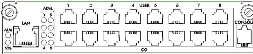
Figure 7-3 AAM1008 Front Panel LEDs
