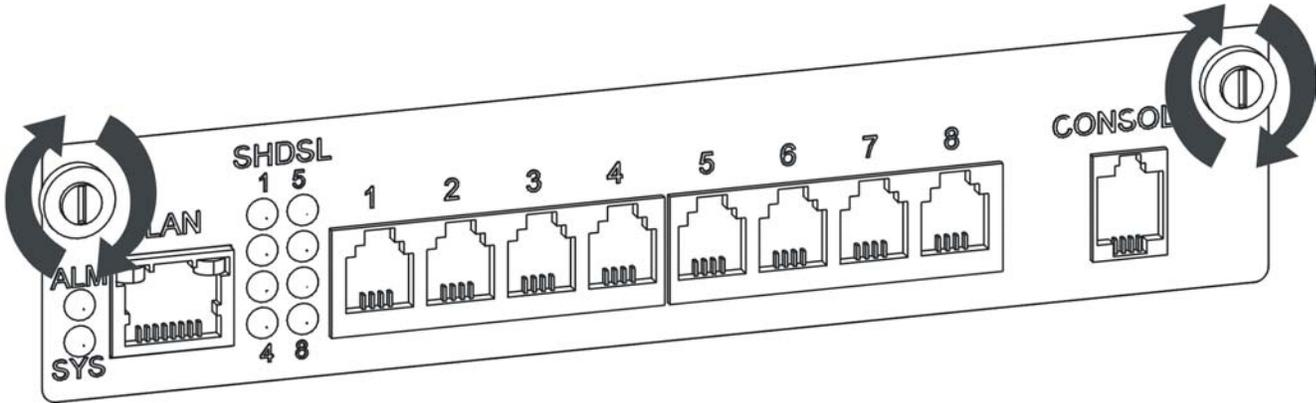
**Figure 5-5 Tighten Module Screws**
