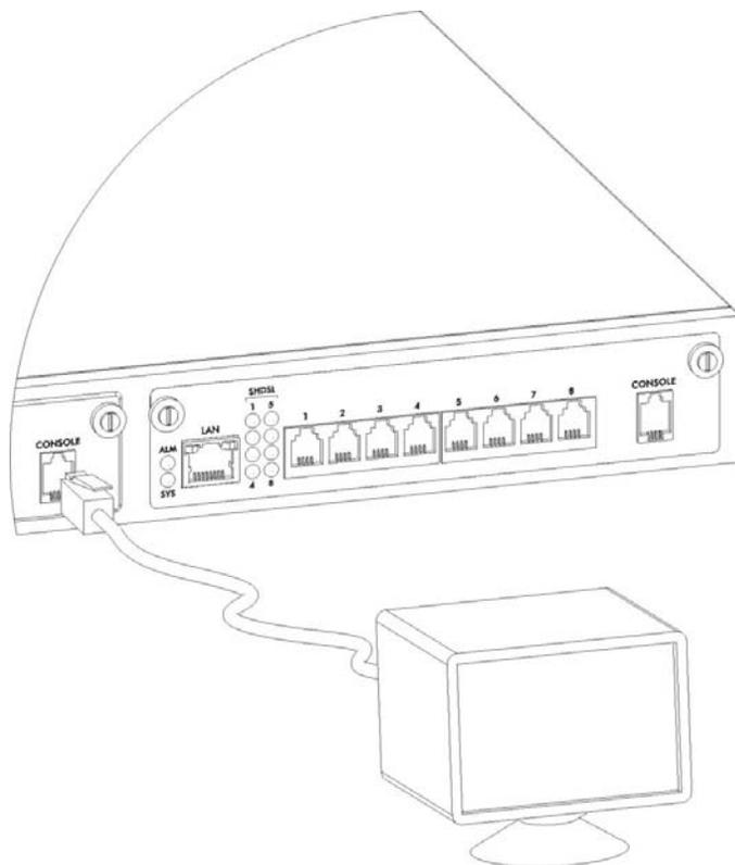
**Figure 6-2 Console Port Connection**
