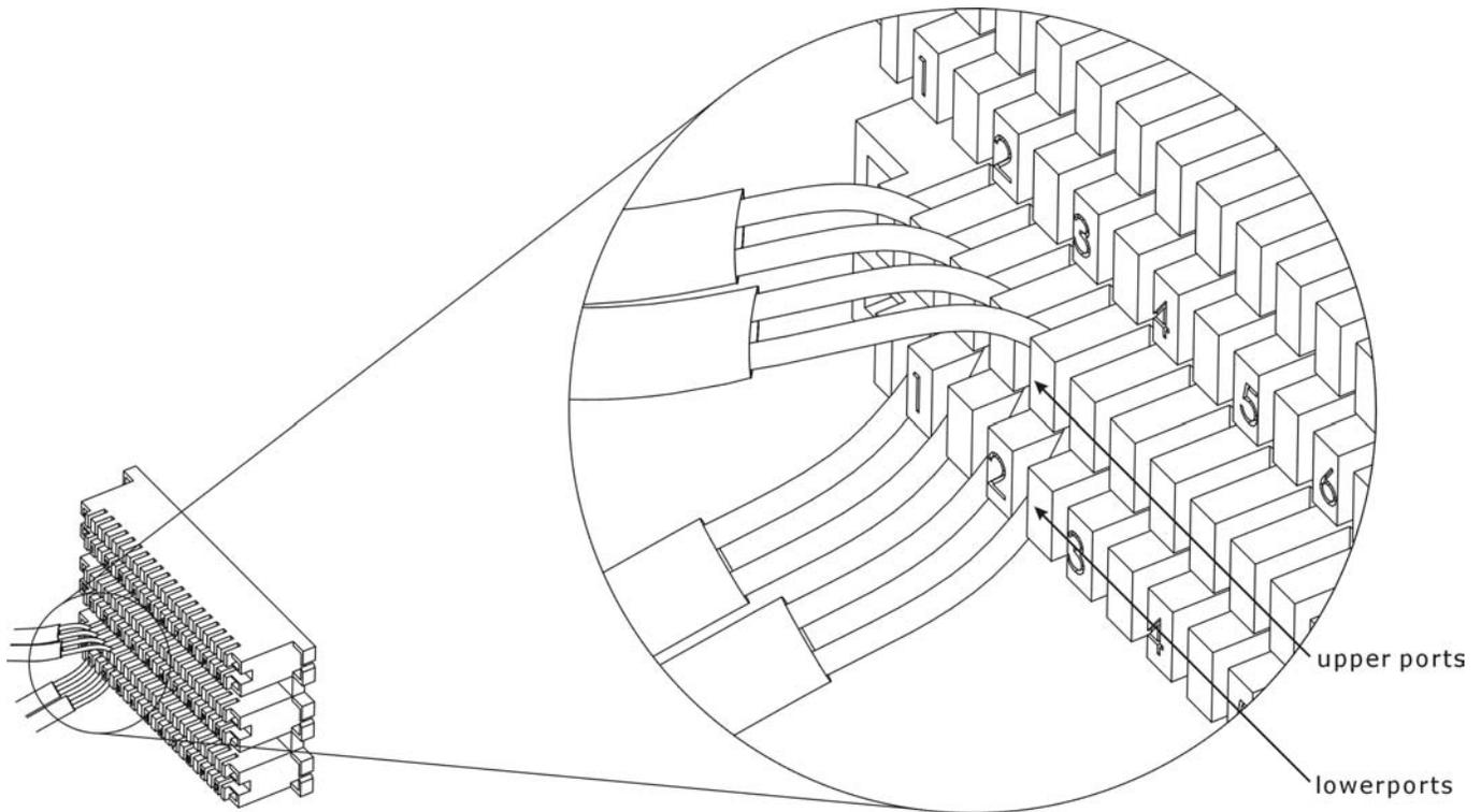
**Figure 6-5 Magnified View of MDF Wiring**
