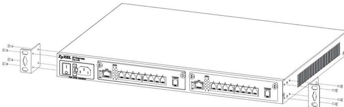
**Figure 4-1 Attaching the Mounting Brackets to the IES-1000**
