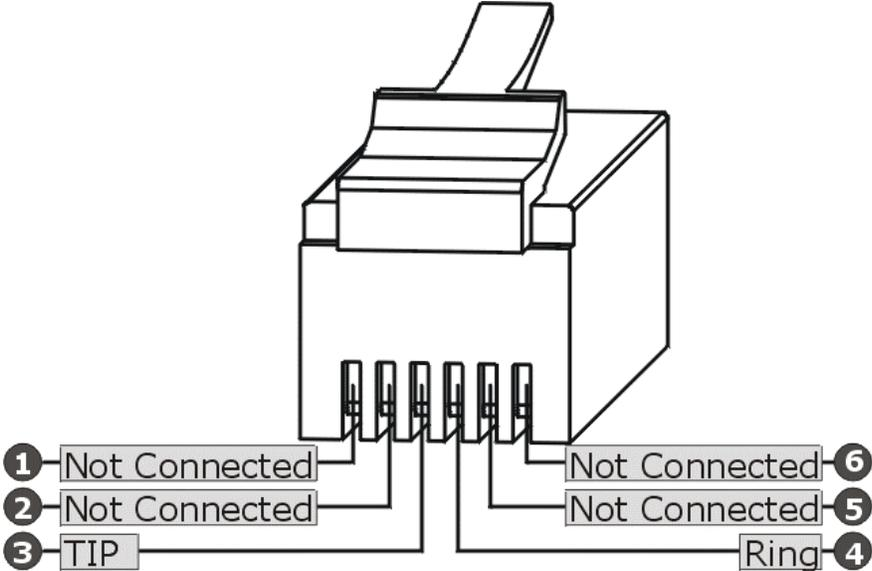
Diagram 4 RJ-11 6P2C (SHDSL Port) Pin Assignments
