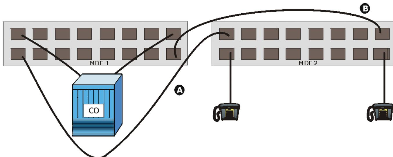
**Figure 6-10 Two Separate MDFs for End-user and CO Connections**
