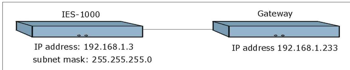
**Figure 33-1 Setting IP Address and Default Gateway**
