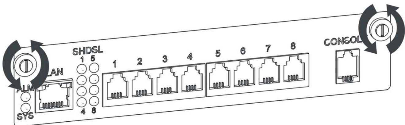
**Figure 5-2 Loosen Module Screws**
