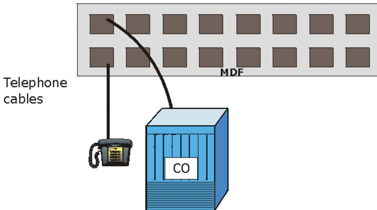
**Figure 6-8 One MDF for End-user and CO Connections**
