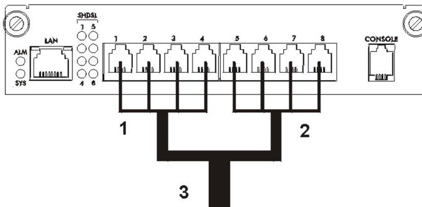
**Figure 12-1 N-wire Mode with Port Bonding Example**
