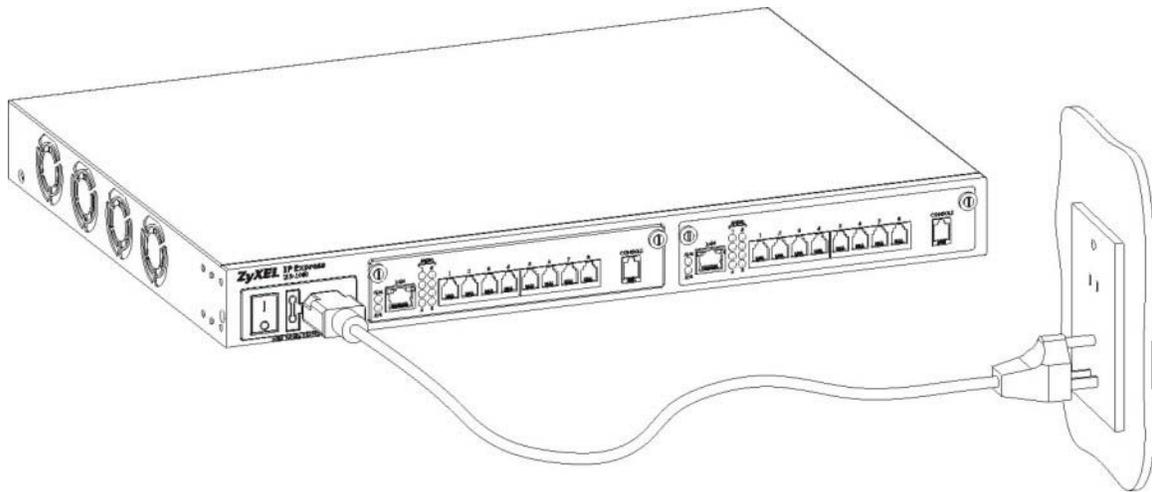
**Figure 6-13 Connecting the Power Cord to the IES-1000 and a Power Source**
