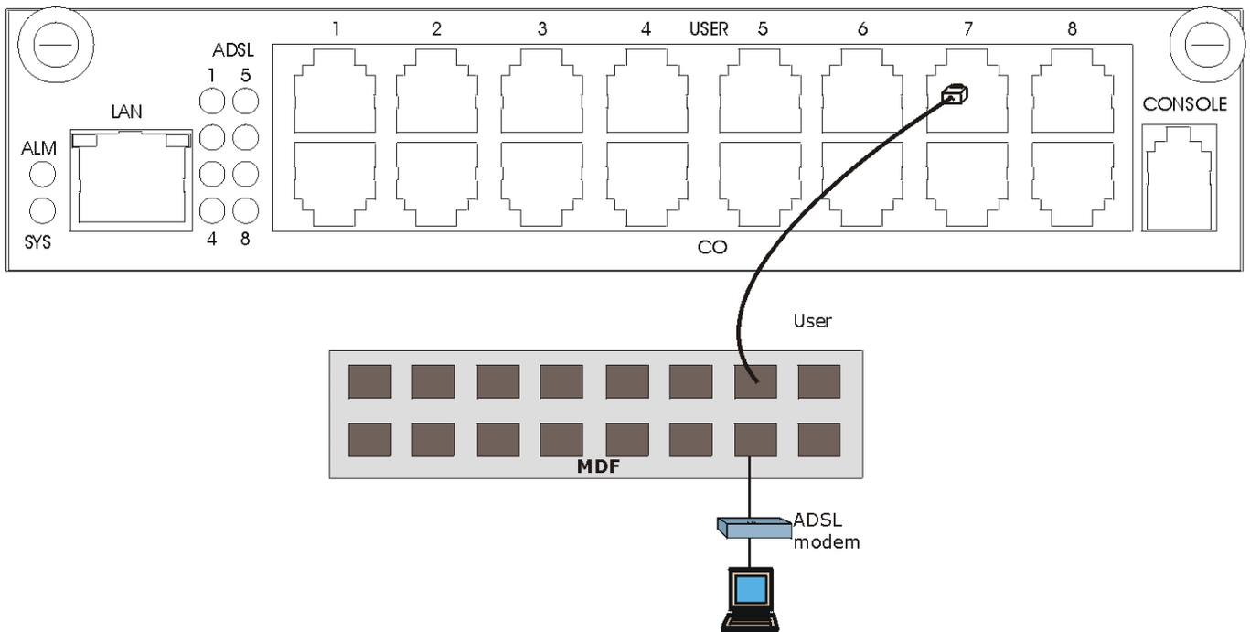
**Figure 6-7 Installation Scenario A**
