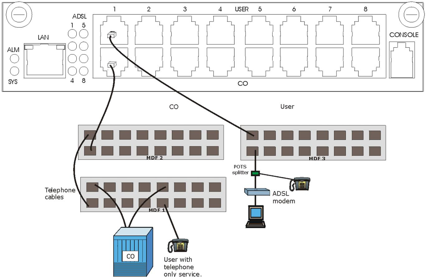
**Figure 6-9 Installation Scenario B**
