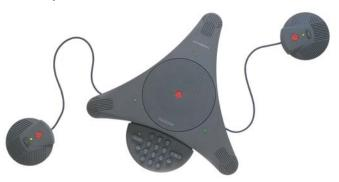
Tabletop console contains all audio processing functions and keypad. Wall module and universal module contain power and telephone line interfaces. Cables consist of 25 ft (7.6 m) connection to tabletop unit and 7 ft (2.1 m) connection to telephone jack.
