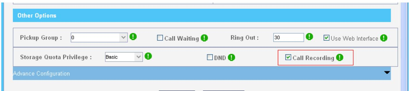
Enable call recording in PBX settings -> Trunks for a trunk, all incoming & outgoing calls through this trunk will be recorded automatically.
