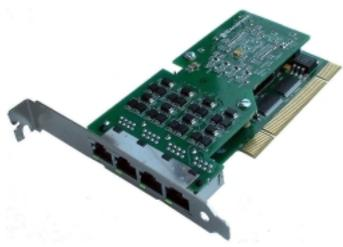
with minimal real-time processor load. This provides optimal performance in demanding environments such as soft PBX/IVR voice applications.
