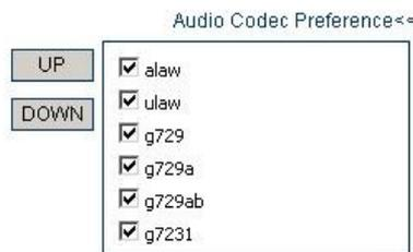
If a compression coding is ticked, it indicates that the compression coding is available. The **UP** and **DOWN** are used to adjust the priority of the selected voice compression coding.
