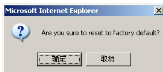
Click OK. All the parameters of the gateway will be cleared and the gateway will automatically restart. After the gateway is restarted, all the settings restore to the factory default settings. This feature can be completed by using the asterisk command. For details about this operation, see the
