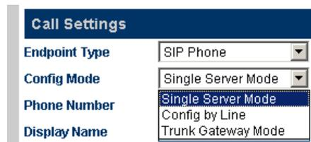
Figure 3-31 Setting Mode in the SIP Terminal
