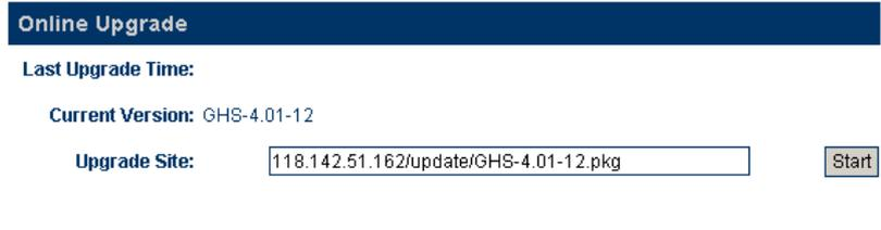
Note: During the upgrading, do not cut off the power. Otherwise, the GoIP will be damaged.
